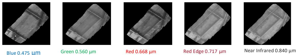
Fig 2. Individual band Orthomosaic from MicaSense RedEdge Sensor
