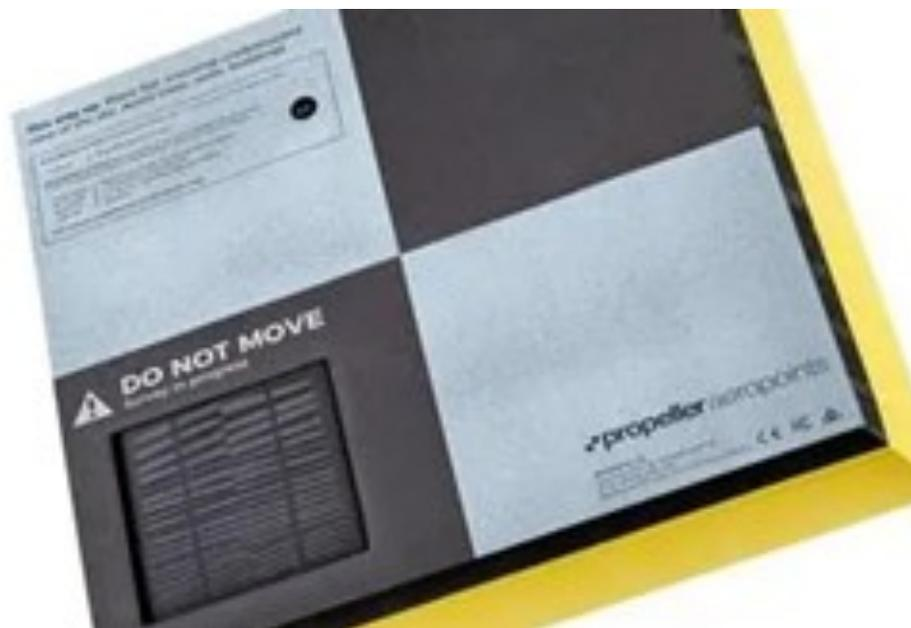
Fig 6. Aeropoint™ GCPs from Propeller Aero.
