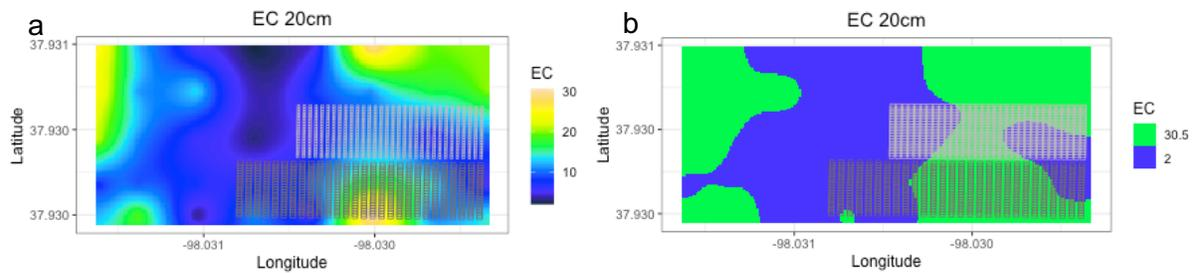
**Fig 1. Kriged (a) and k-means cluster contour (b) maps for 0-20cm depth EC from the P4000 at 21RNS with PYN and YT plot map overlays. Number of color clusters in the cluster map were determined by k-means clusters and the values for the cluster color represent the median value of the cluster for ECa.**
