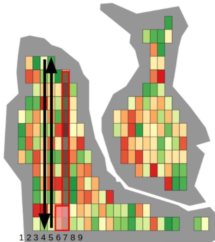
Fig 1. Example of an optimal prescription map. The arrows indicate the path the applicator takes along the plots. The shaded rectangle shows an example a subpopulation based on a strip of cells in the field. The shaded square is an example of a group of two ending and starting cells of consecutive strips to form overlapping subpopulations.
