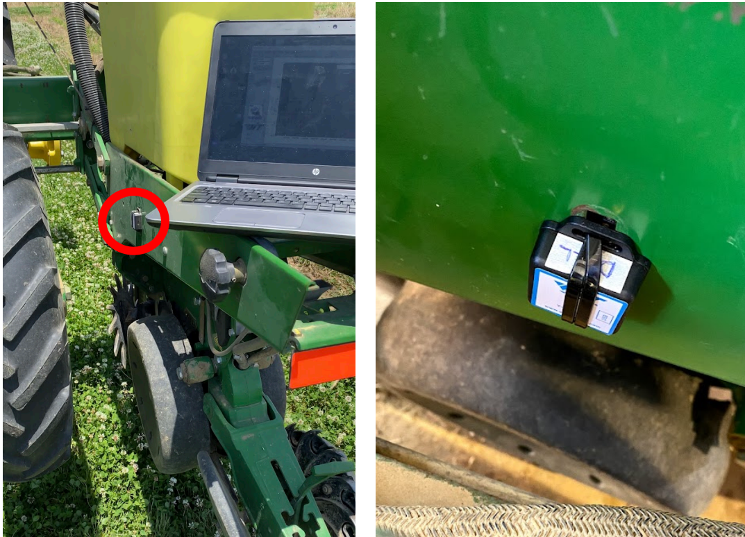
Figure 2: Accelerometers installed on the planter. The red circle indicates the location where the accelerometers were installed.
