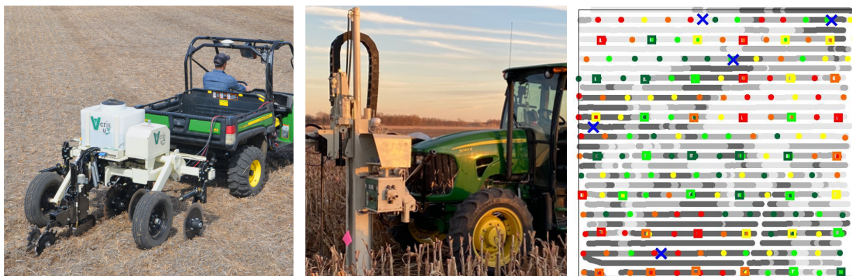
Figure 5 and 6. Veris U3 (left) and P4000 (center). Figure 7. Example map showing blue X's that mark sensor probe calibration location. Squares mark .4 ha grid samples, sensor probe insertions, and location of sensor probe estimates of SOC.
