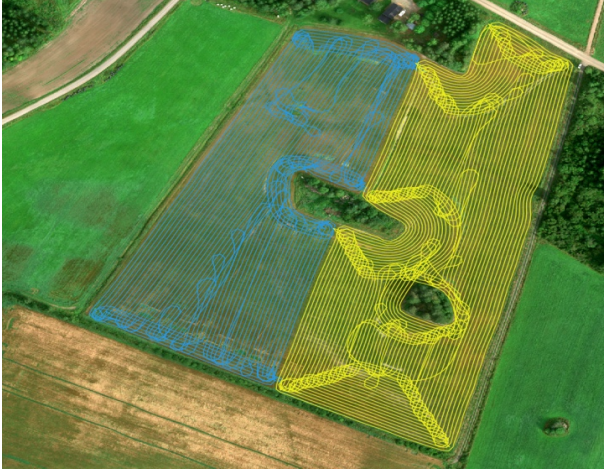
Figure 4. Route map during the sowing process. Automatic steering on the left, manual steering on the right.
