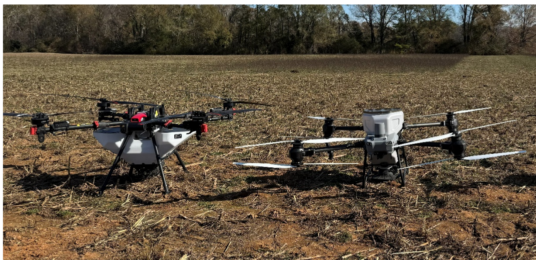
Figure 1. DJI Agras T50 (left) and XAG P150 drones used to test different metering and spreading systems in this study.
