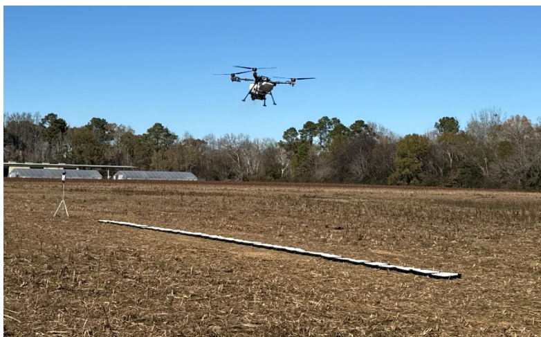
Figure 2. Illustration of collection pans placed within the application area and perpendicular to the drone pass for assessing the distribution uniformity of cereal rye across the swath.
