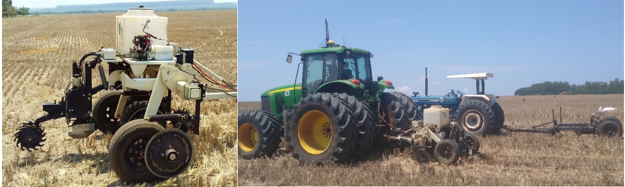
Figure 1: Detail of ECa mapping device VERIS U3 (A) and both EC rigs being tested, VERIS3100 in the front and DC-based prototype in the back of the picture (B).
