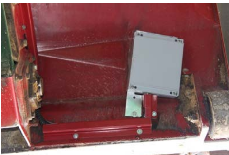
Figure 3 near infrared sensor head (left outside, right in side)
