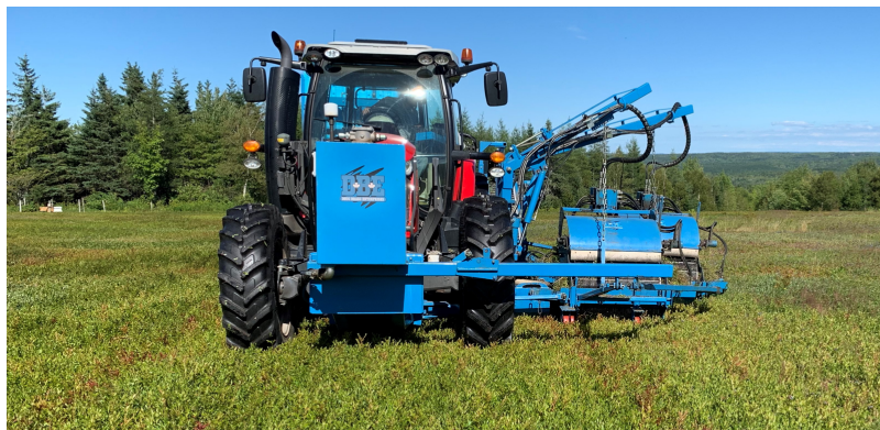
Figure 2: Doug Bragg Enterprises mechanical harvester mounted on a farm tractor.
