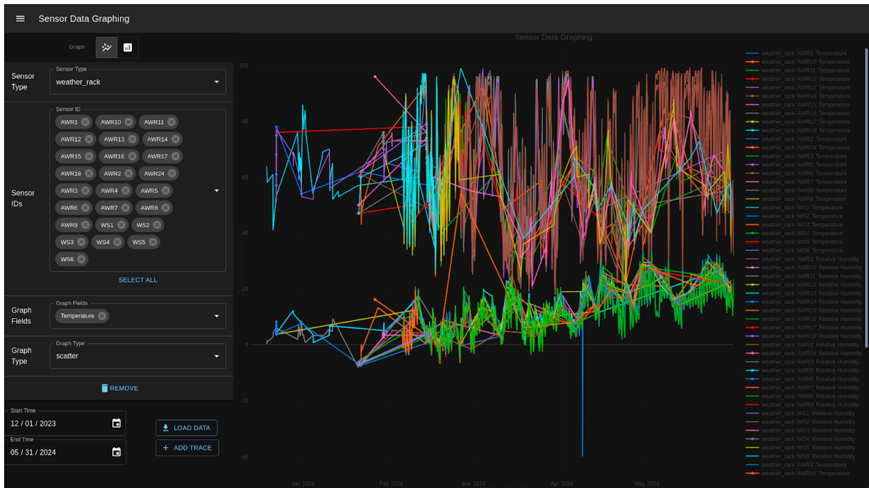
Plot of 264,162 points rendered live in the browser as part of the sensor data graphing page.
