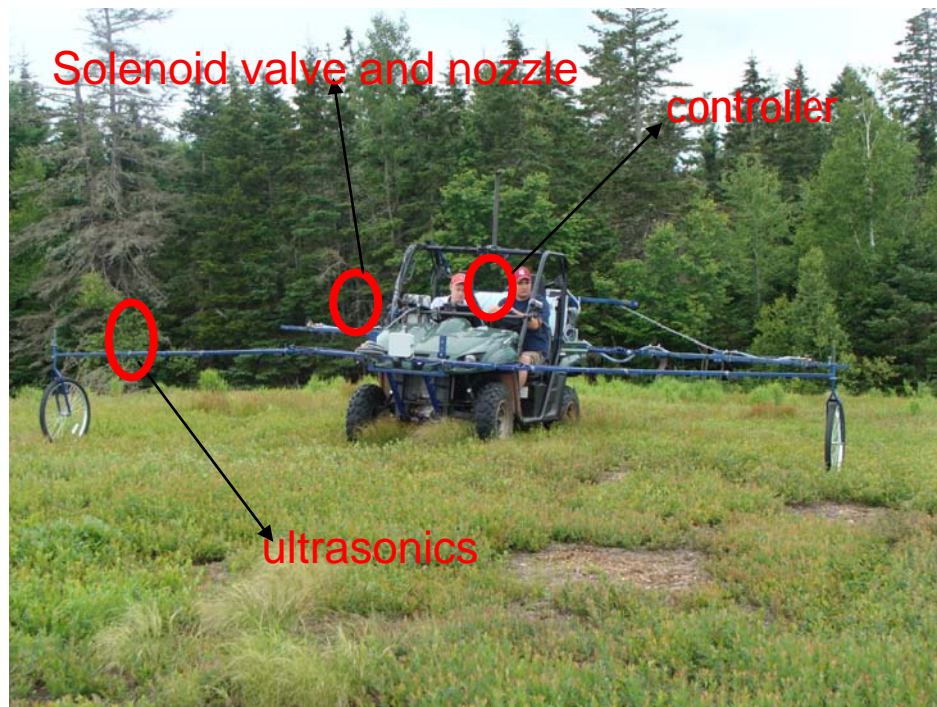
Fig.1: An automated variable rate sprayer for spot- application of agrochemicals.
