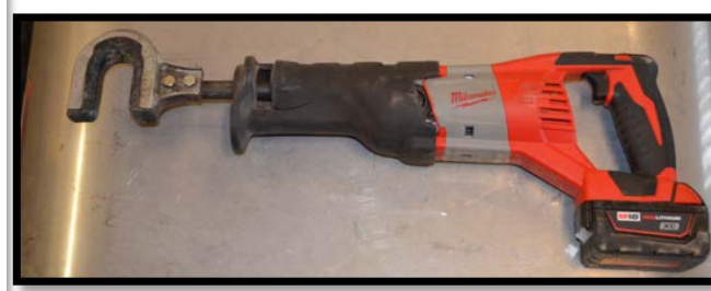
Figure 5. Hand-held high frequency linear actuator (right) used for limb shaking ‘Fuji’ and ‘Granny Smith’ apples.
