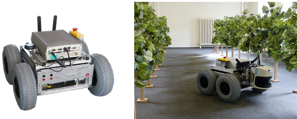
Fig. 4. The simulation platform VolksBot, running on an indoor test track.
