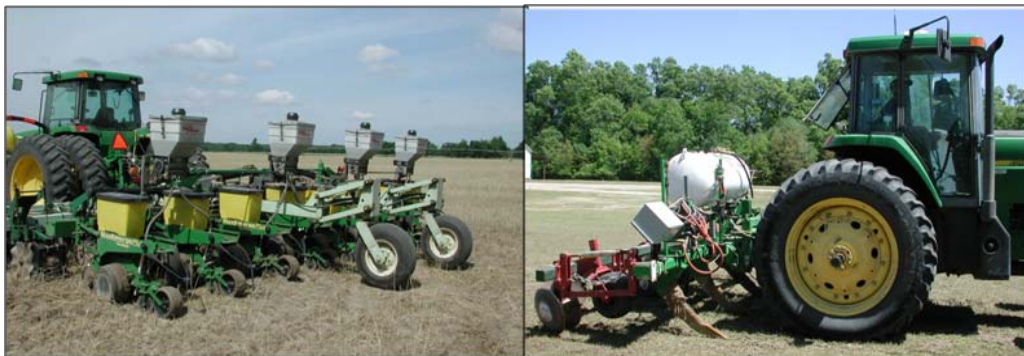
Figure 1. An 8-row SNP system for granular nematicide application (left) and a 4-row SNP system for fumigant nematicide application (right).
