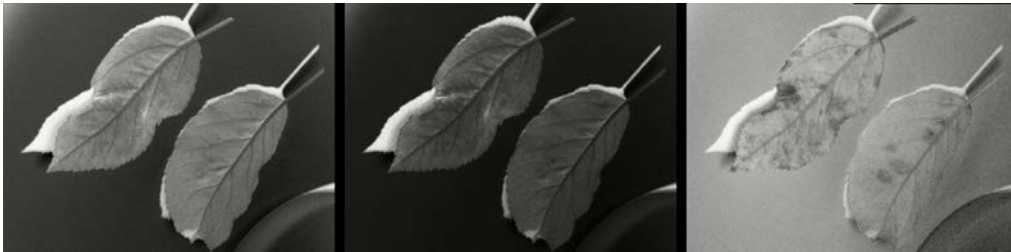
Figure 3. Images from adapted RGB camera. Comparison of indexes for best contrast of sick spots, from left to right: NDVI, RVI, MNDVI. The latter is best. (Note: The white parts under the leaves are shadows.)
