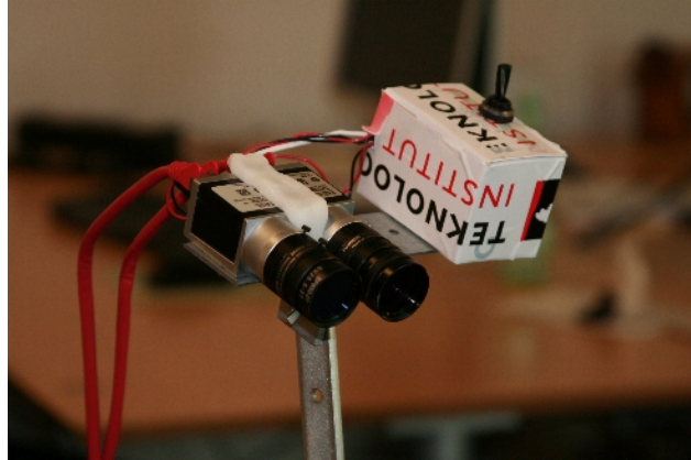
Figure 2. Two camera system with red plus polarizer filter on one and near -infrared on the other.
