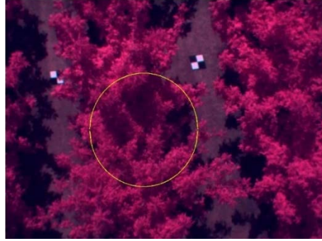
Fig. 1. The yellow circle illustrates the IR sensor FOV as seen in a typical image of a walnut canopy. The checkered targets were used for GPS reference.
