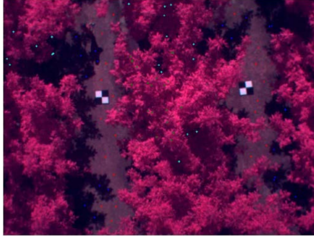
Fig. 2. The pixels identified by colored dots were determined to be representative of each class of material: sunlit leaves, shaded leaves, sunlit soil, and shaded soil.
