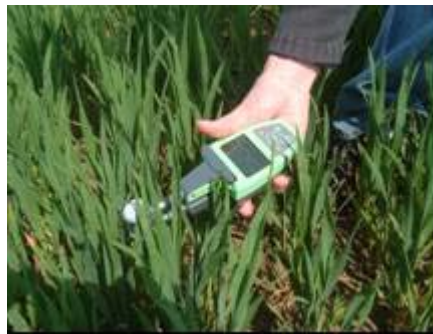
Fig. 1. Picture of Dualex leaf-clip while assessment on wheat.
