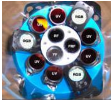
Fig. 2. Front view of Multiplex optical head with LED sources (6 UV & 3 RGB) and three detectors in the middle (YF, FRF, RF).
