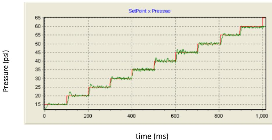
**Fig. 6.** Pressure readings after flow valve PID control, red set point, green valve response.
