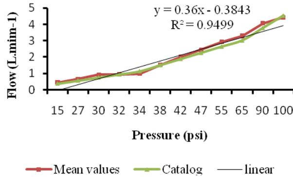
**Fig. 5.** Varitarget calibration curve
