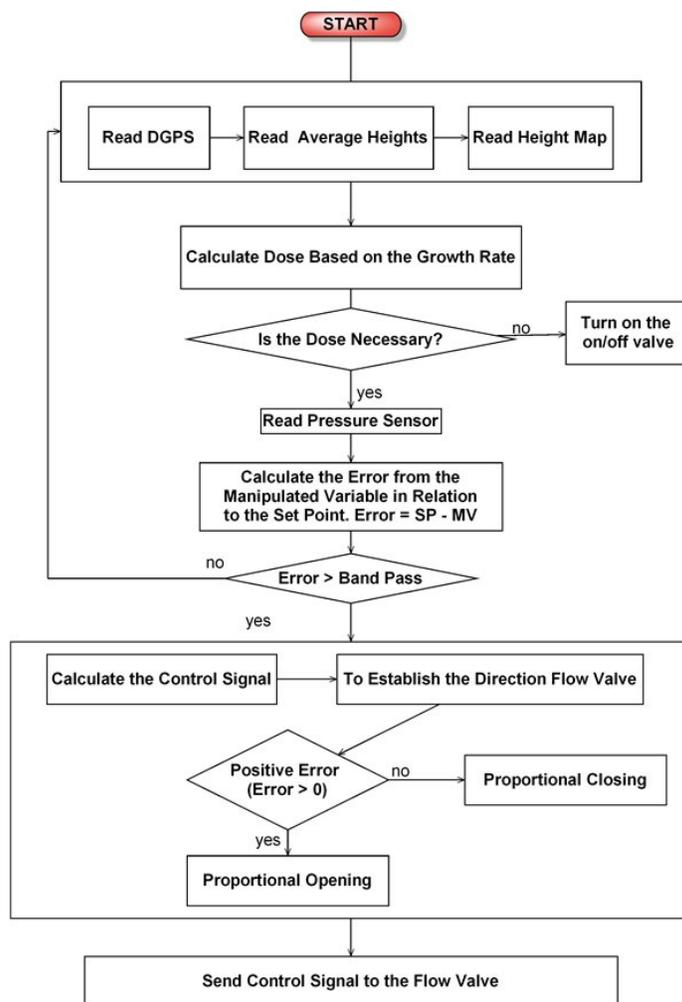
**Fig. 4.** Flow Chart of Pressure valve Controller Software
