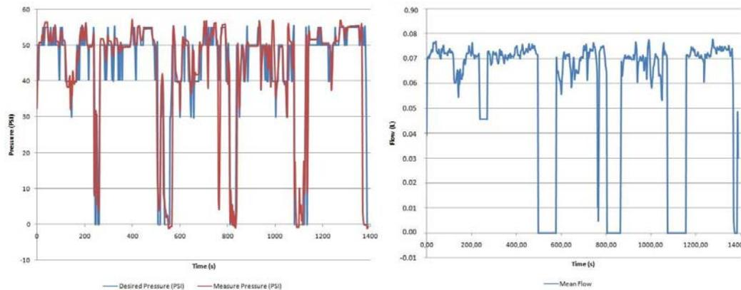
**Fig. 9.** Desired pressure and measure pressure during a simulation period (a) and the mean flow over the same period (b) at sprayer forward speed of  $2.5 \text{ m.s}^{-1}$ .
