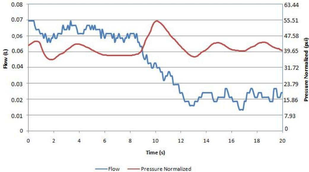
**Fig. 10.** Flow and pressure in a 3 nozzles system when the flow in 2 nozzles was obstructed.
