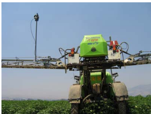
FIGURE 1. IR scanner mounted on high pass sprayer.
