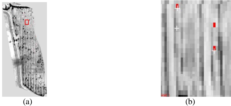
Fig. 14. Spectral unmixing method applied on E1 (west grove site). (a) Spectral unmixing applied on MNF transformed image of Fig. 12(a). Red pixels indicate infected trees which were matched based on high abundance threshold value. (b) The white cross-hair on the enlarged rectangular subsection of (a) indicates ground truth location for infected trees.
