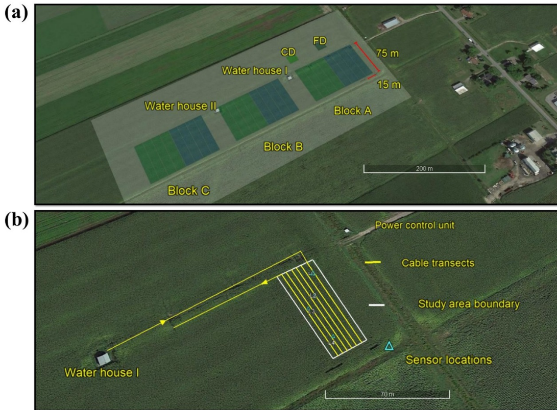
Fig. 1 (a) Shows the study area which consists of three main blocks A, B and C. Blue and green rectangles within the main block are sub plots (15×75 m) free drainage (FD) and controlled drainage(CD). Two water houses facilitate the measurement of drainage volume from each sub plot. (b) shows the fiber optic cable configuration in the field. Cable connected to the DTS instrument starts from the water house I and runs through two subplots at three depths (0.05, 0.10 and 0.20 m), blue rectangles show the locations of 5TE sensors used for calibration and validation.
