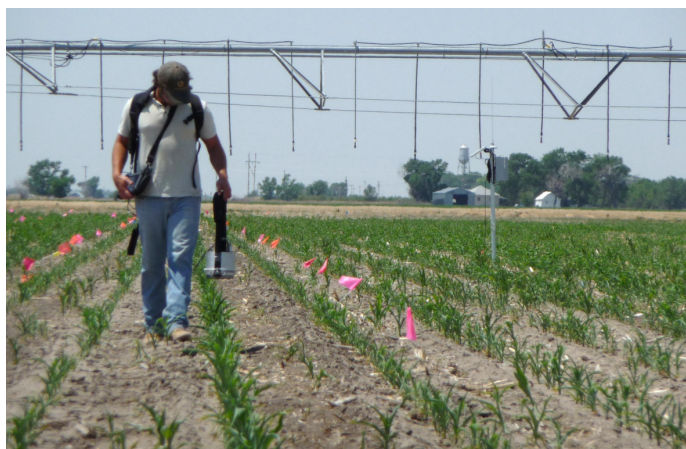
Fig. 1. Mobile acquisition mode of Multiplex®3 fluorescence sensor over maize canopy in field.
